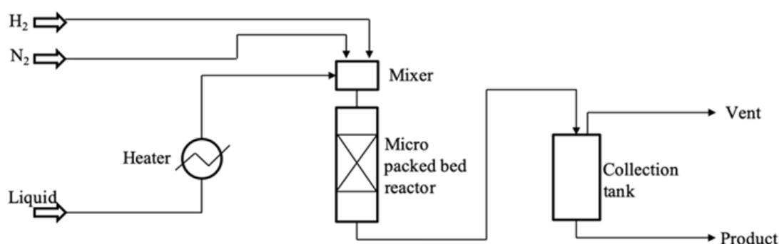
Figure 2. Micro-packed bed hydrogenation reactor process flow chart.
