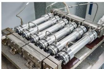
Silicon Carbide Tubular Reactor
