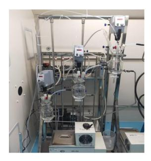
Figure 7 A three-stage MSMPR crystallizer.
