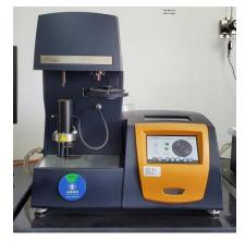
Figure 3 PLM with hot stage and DSC used for sublimation property study.
