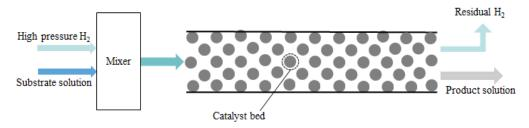
Figure 1. Micro-packed bed reactor.
